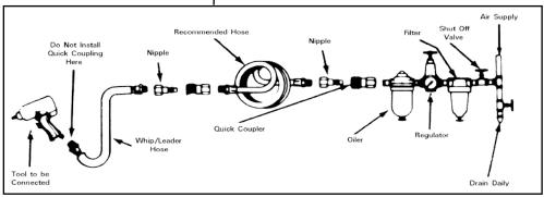
supply and run tool slowly for a few seconds to allow air to circulate the oil. If tool is used frequently lubricate on daily basis and if tool starts to slow or lose power.
